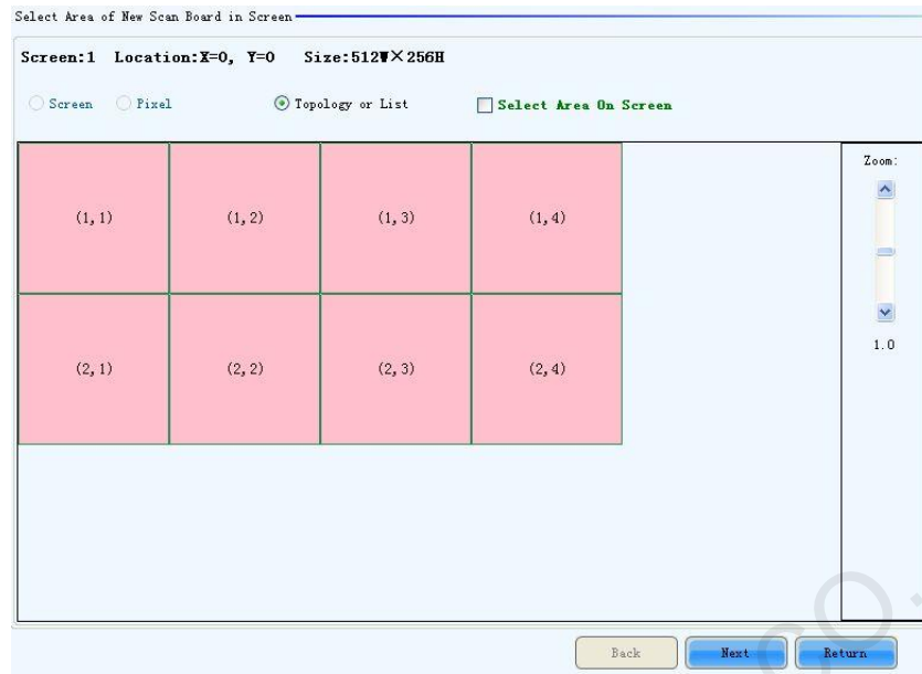
Figure 5-51 The page for specifying the working area of the new receiving card
